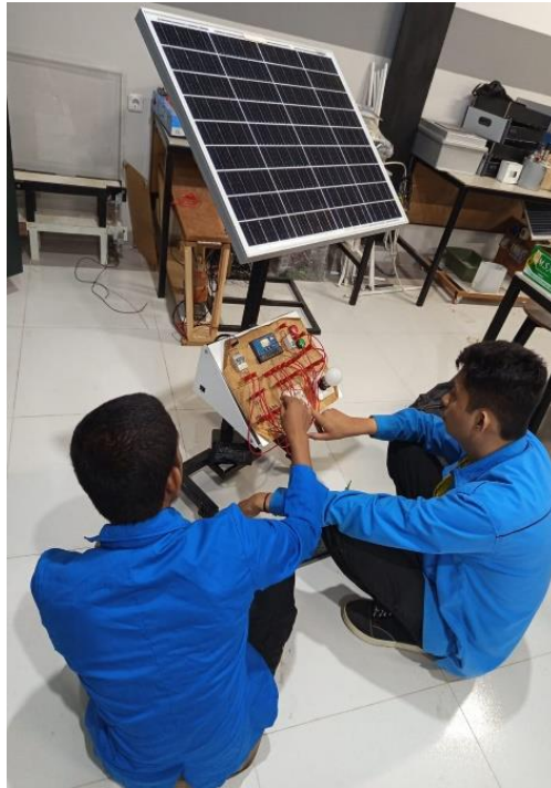
Gambar 3. Proses Pengujian PLTS 100 WP
